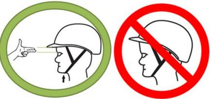
Position the helmet so it is even and level. Two finger widths should be between the top of the eye and the helmet. Avoid the helmet been pushed back over your head or low over your eyes.
