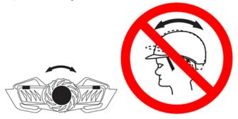
Place the helmet on your head in the correct position (see 6) and turn the dial on the adjustment mechanism so the helmet fits snugly or comfortably firm. The helmet must not be able to freely move backwards and forwards on the head. If the helmet size does not match your head size or there is insufficient adjustment for it to properly and comfortably fit your head, do not use and select a helmet size that properly fits your head.
