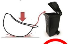
Helmet may be seriously damaged from receiving an impact to the point that it is no longer adequate to protect the head against further impacts and that damage may not be visible to the user. A helmet that has sustained an impact or severe blow, must be destroyed and replaced
